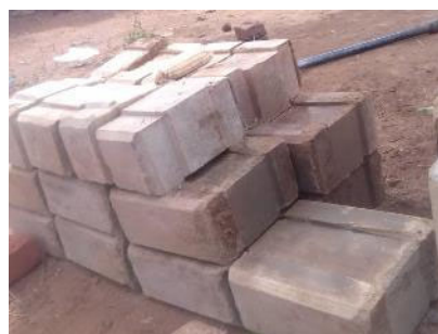
Prototype Inter-locking Soil Stabilised Blocks to be used in construction
